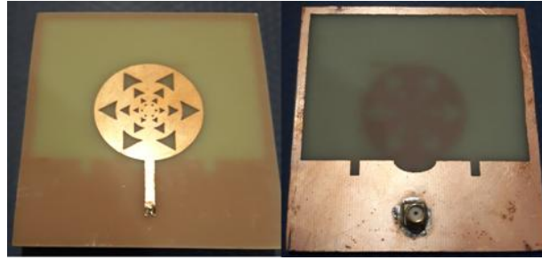
Figure 3 Fabricated Circular shaped fractal slot antenna
